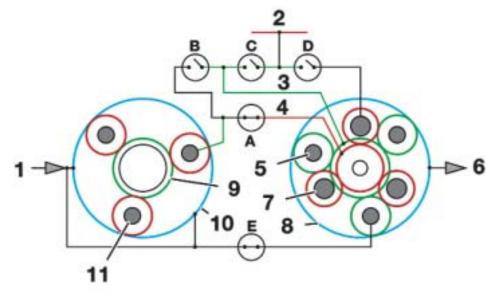
**Power Flow in 5th Gear:** Drive clutches B and E are engaged in 5th gear. The sun gear 2 (3) in the double planetary gear train is driven by clutch B and the planet carrier of the double planetary gear train by clutch E. Together with the double planet carrier, the long planet gears and the short planet gears drive the internal gear 2 in the direction of engine rotation. *This results in a gear ratio with a slight overdrive*.
